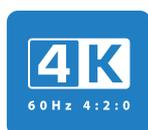
The 4K data rate varies depending on the requirement for differing frame rates, colour depths, and colour gamuts. 4K 60Hz 4:2:0 requires 10.2Gbps of data transfer capability.
