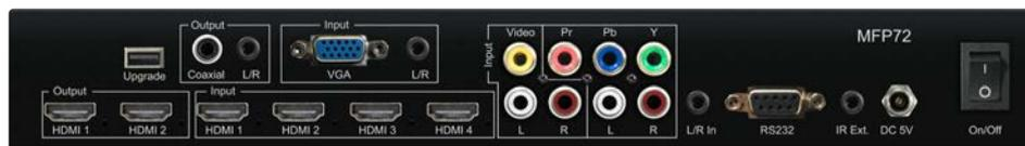
Our MFP72 is a multi-format presentation switcher with in-built video scaling, audio embedding, de-embedding and EDID management. The MFP72 works in 2 modes, first as a 7 input dual output switcher, alternatively each output can work independently with output 1 routing the 4 x HDMI inputs only and output 2 switching all 7 video / audio inputs. With control of the switcher using the front-panel push buttons, IR remote control or RS-232.
