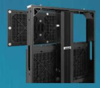
Modules are magnetically captive to the frame allowing for flexible mounting; hung, wall mounted, fixed frame mounted, or stacked.
