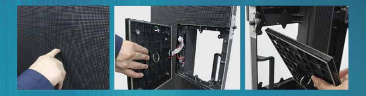
Uslim features a unique push and pull design between module and cabinet. When it comes to maintenance, complete front and rear service is available. Modules are magnetically captive to the frame allowing for flexible mounting; hung, wall mounted, fixed frame mounted, or stacked.
