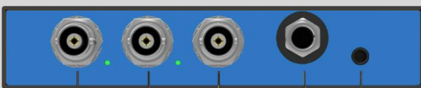
SDI In Alt SDI In SDI Loop Out AES/EBU In Analog Audio In
